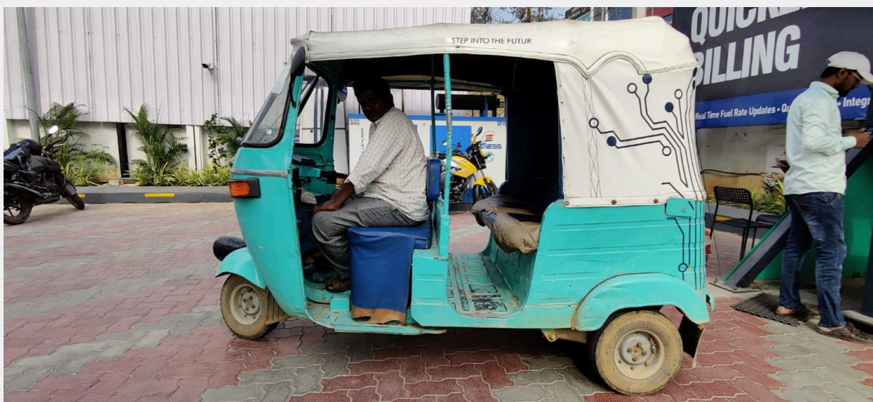
FIGURE 5 | A retrofitted e-auto at a battery swapping station in Hyderabad
