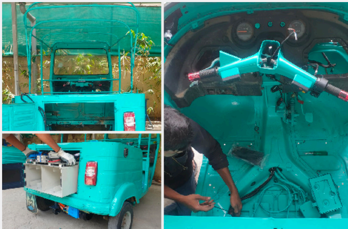
FIGURE 6 | A conventional auto-rickshaw being converted into an e-auto with a retrofit kit
